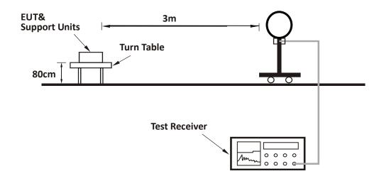
For Radiated emission 30MHz to 1GHz:
