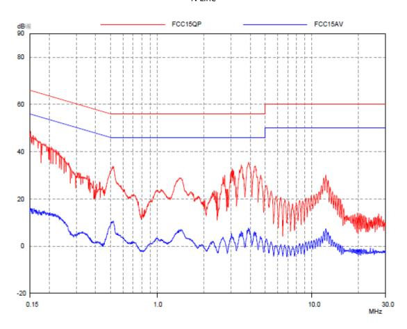
Remark: 1. Correct Factor = LISN Factor + Cable Loss, the value was added to Original Receiver Reading by the software automatically.
