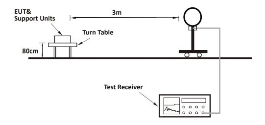
For Radiated emission 30MHz to 1GHz:
