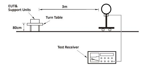
For Radiated emission 30MHz to 1GHz:
