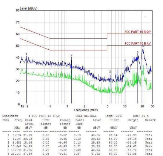
Remark: Level = Read Level + LISN Factor - Preamp Factor + Cable Loss
