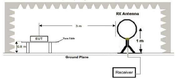
(2) Radiated Emission Test-Up Frequency 30MHz~1GHz
