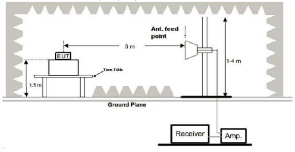
(3) Radiated Emission Test-Up Frequency Above 1GHz
