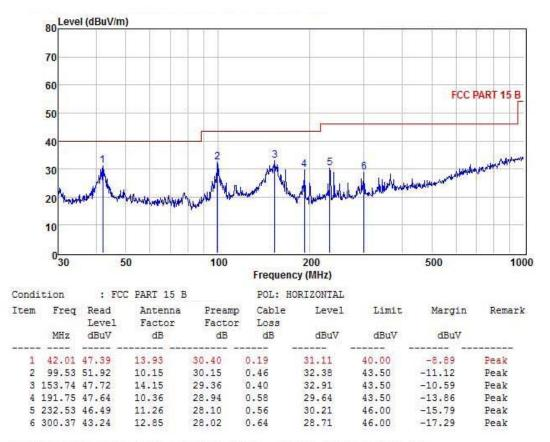
Remark: Level = Read Level + Antenna Factor - Preamp Factor + Cable Loss
