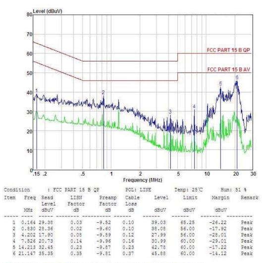
Remark: Level = Read Level + LISN Factor - Preamp Factor + Cable Loss
