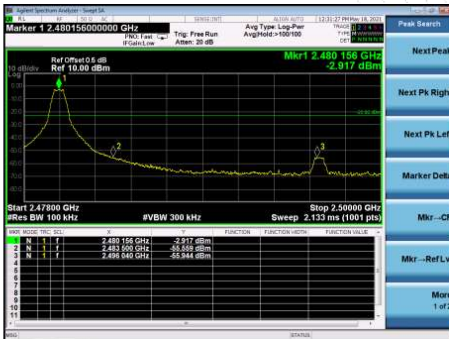
GFSK: Band Edge, Right Side
