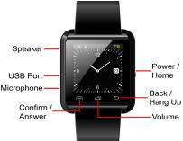
**POWER/HOME**: Press and hold to power on/off. Press once to turn the screen on, or to return to standby.
