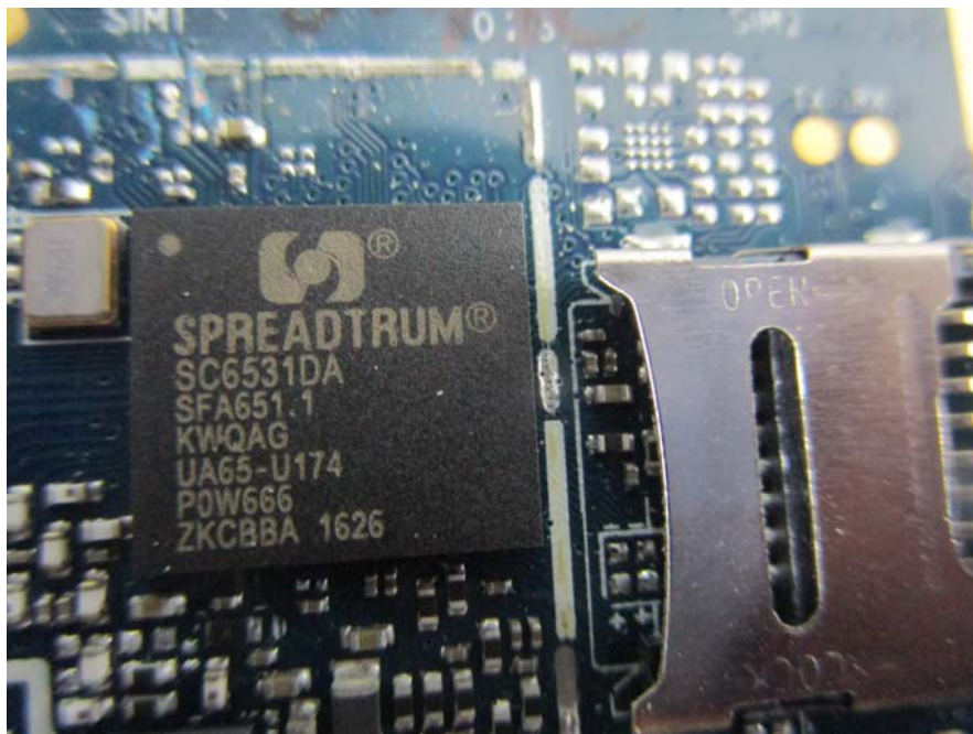
EUT – Main Chip View
