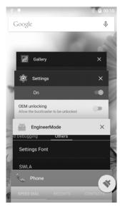
Your tablet supports multi-task operation, allowing you to switch between different applications easily. To view this screen, press and hold the Home button. From here, you can switch to a new program by pressing the corresponding screen. To close a program, swipe its screen left.
