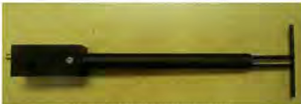
Figure 1 – MVG COMOSAR Validation Dipole
