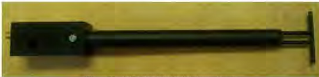
Figure 1 – MVG COMOSAR Validation Dipole
