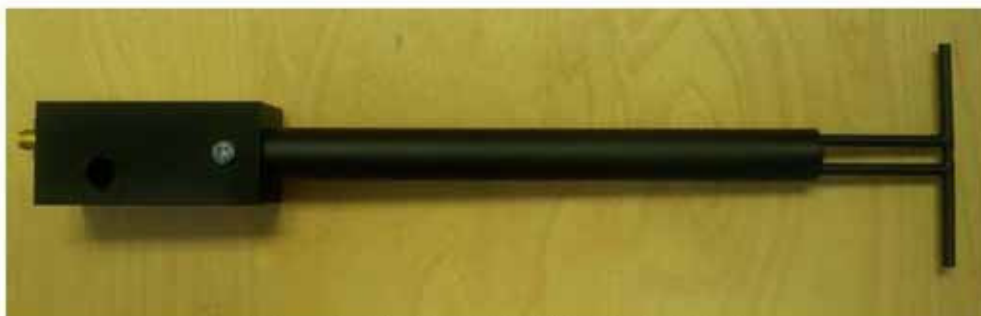
Figure 1 – MVG COMOSAR Validation Dipole
