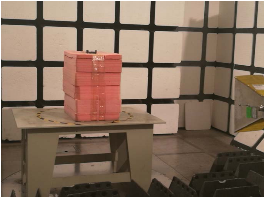
Radiated Emissions View (Above 1 GHz)
