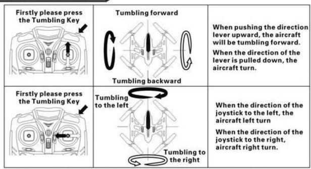
Tips: Please fly the aircraft to the height of 1.5meters or above, and then make the aircraft tumbling.
