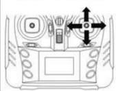
When entering "One-key Return Mode", simply pushing the Direction Lever toward either direction(forward or backward or to the left or to the right) can exit from the "One-key Return Mode".
