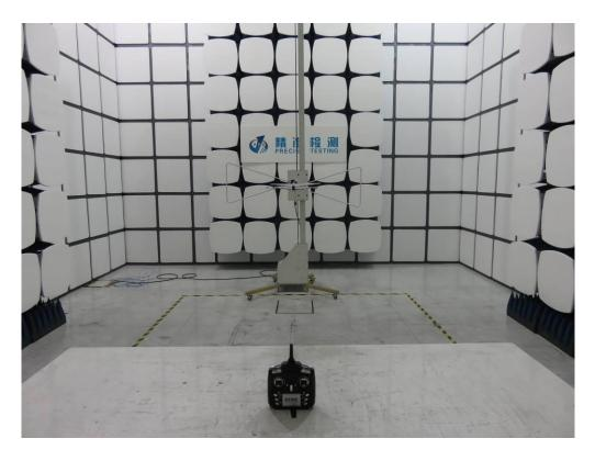
RADIATED EMISSION TEST SETUP ABOVE 1GHz
