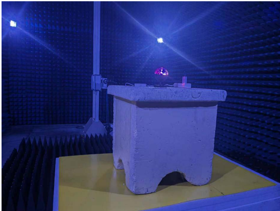
Photo of Radiated Emission Measurement Above 1GHz
