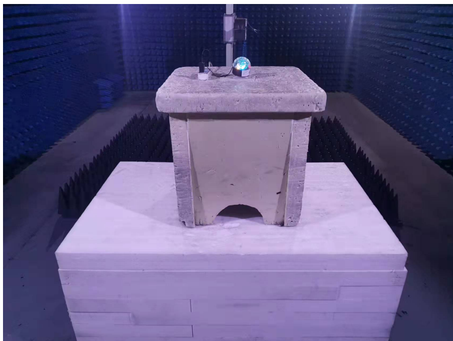
Photo of Radiated Emission Measurement (Above 1G)
