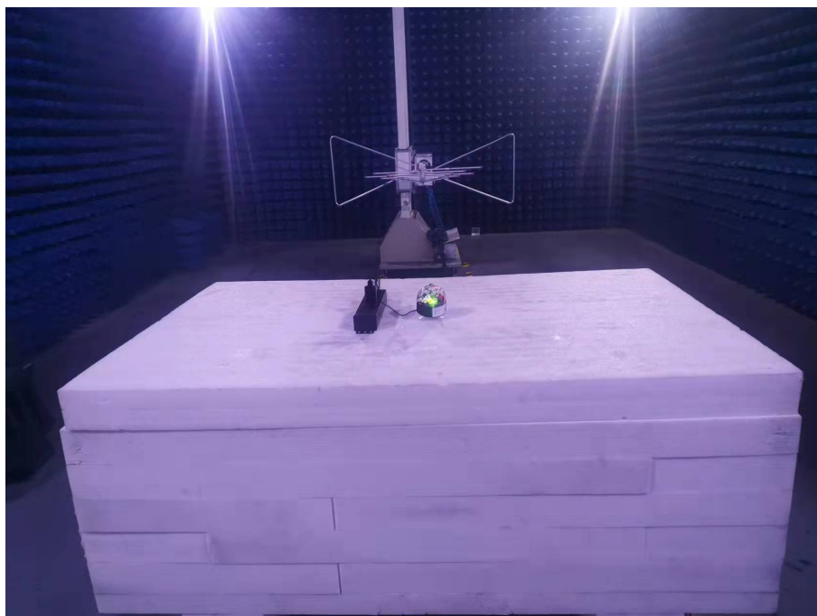
Photo of Radiated Emission Measurement (Above 1G)
