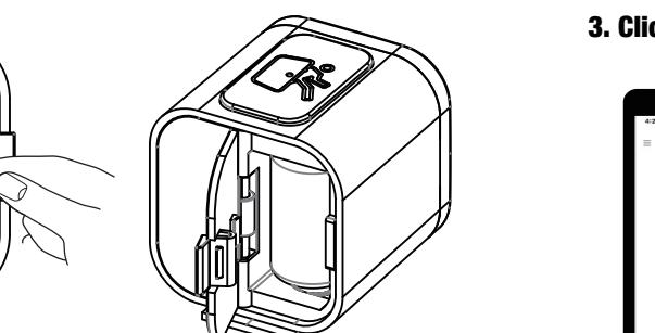
1. Open the cover by pressing the battery cover slightly.
