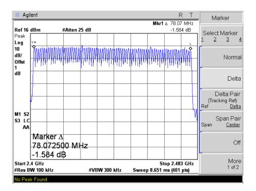
For GFSK mode Channel Spacing (Low CH=1MHz)
