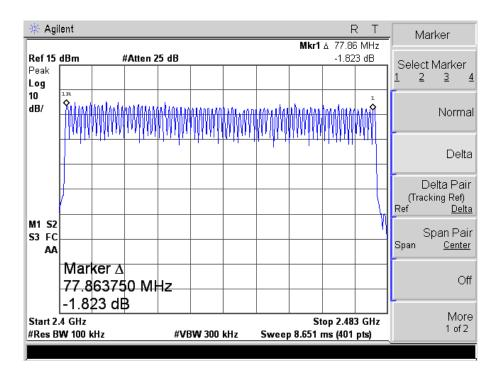
For GFSK mode Channel Spacing (Low CH=1MHz)
