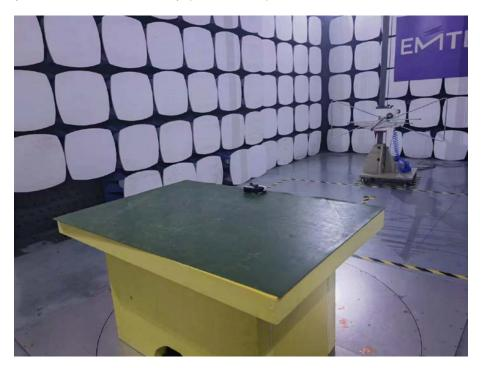
Spurious Emission Test Setup (Above 1GHz)
