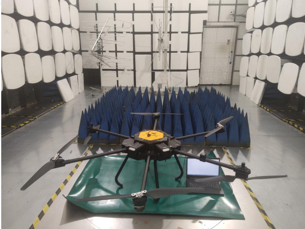
Radiated Emissions Measurement (Below 1GHz)
