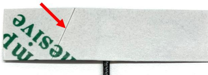
1. Find cut line on flex back side
