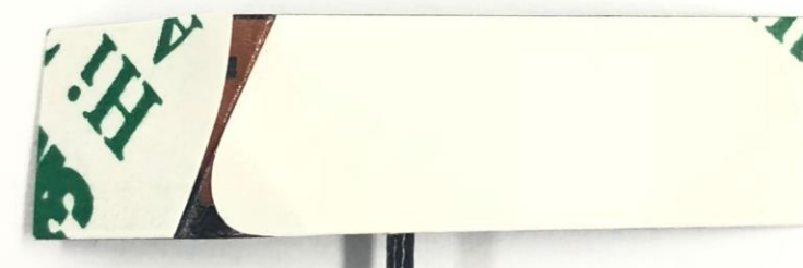
2. Bend flex slight along cut line
