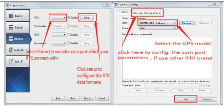
Above picture is configure the device sample, and the Echo sounder pleas select the "Internal port" and tick "Enable"
