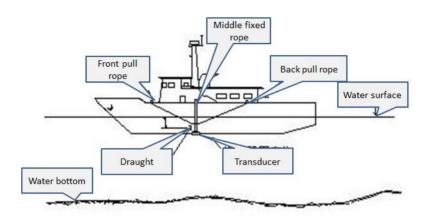
The position of the fixed transducer is best selected next to the middle side of the hull, avoiding the noise interference of the hull as far as possible, and then fixing it by pulling the rope at the front, rear and bottom.
