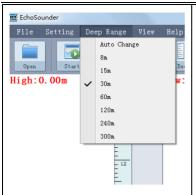
Depth range is important for auto survey mode, and you need to select the correct range to let SOUTH echo sounder adjust the sounding parameters automatically.
