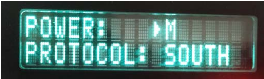
The fourth display interface: the above listed adjusts the radio power. L represents low power. M represents medium power. H represents high power. The following is the tuner protocol interface. (This interface press the confirm button to enter the page turning interface)
