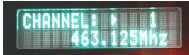
The third display interface: interface of adjusting the radio channel
