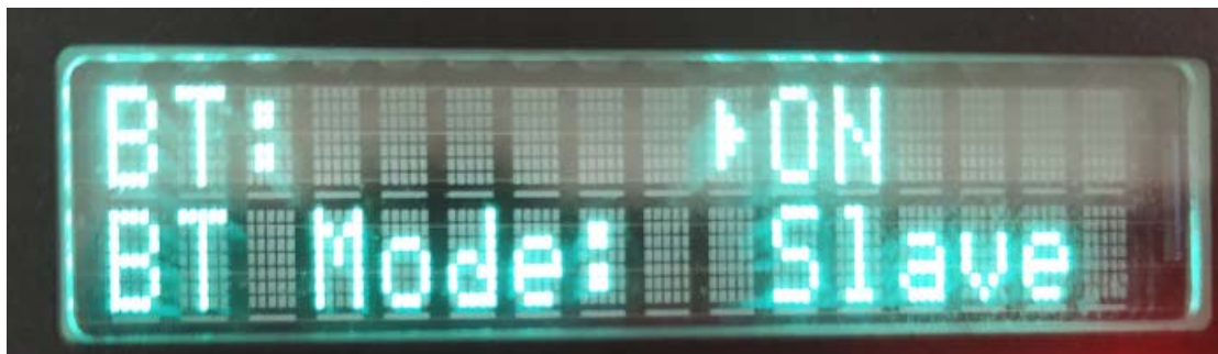
The fifth display interface: the above listed is Bluetooth switch . The following is Bluetooth mode: Slave mode and Master mode.
