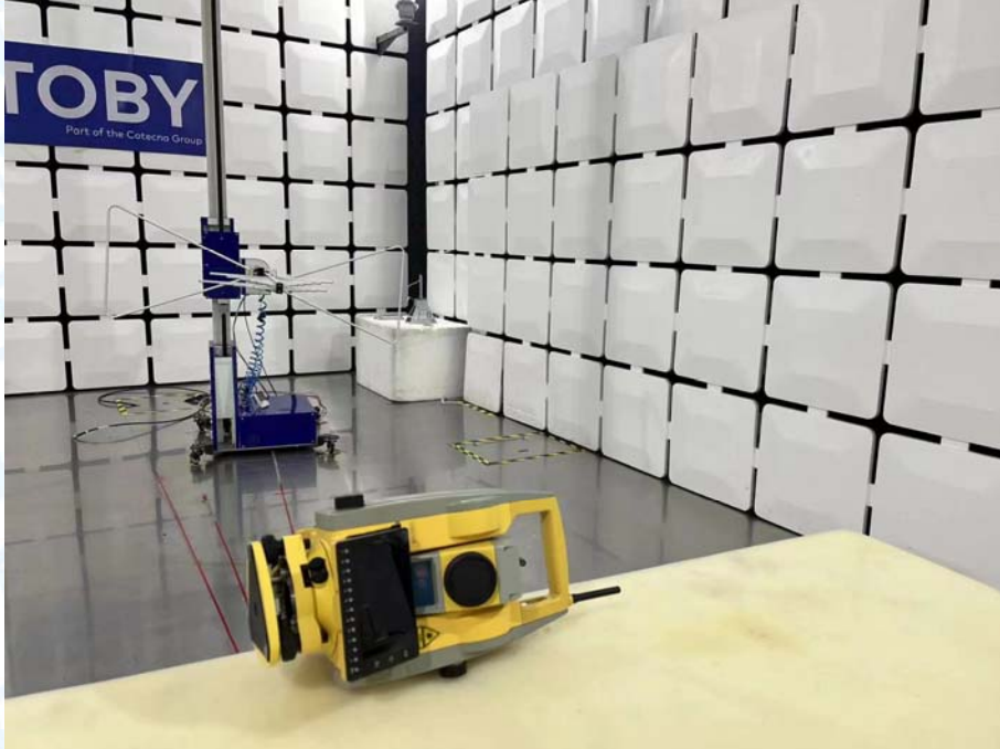
Photo of Setup for Radiated Emission (30MHz~1GHz)
