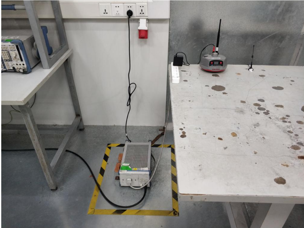
Photo of Conducted Emission Measurement
