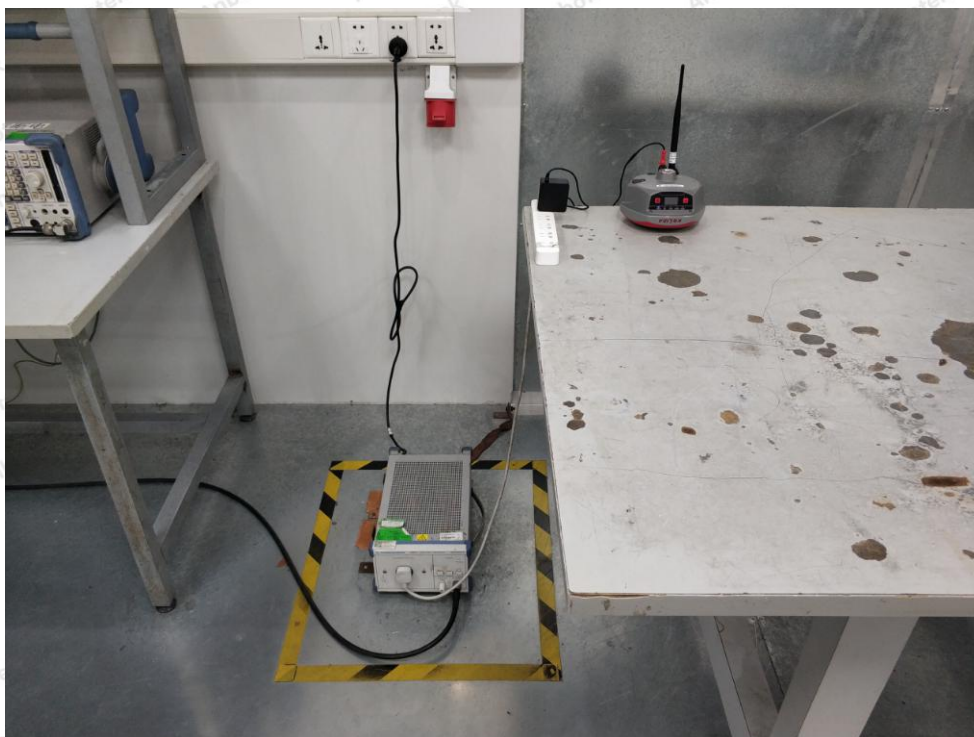
Photo of Conducted Emission Measurement
