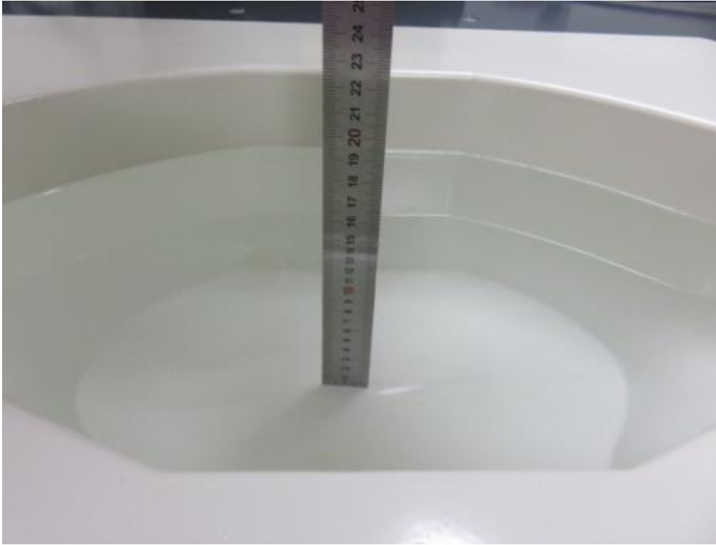
Photograph of the depth in the Body Phantom (835MHz, 16.1cm depth)
