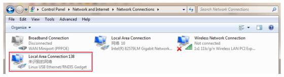
However, sometimes the computer cannot detect the receiver by USB network interface because there is something wrong with acquiring IP automatically, therefore, we need to do something to avoid such problem, that is to set a fixed LAN IP for the connection:
