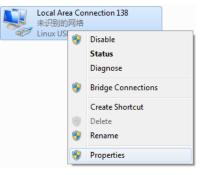
Then double click on Internet Protocol Version 4 (TCP/IPv4) option or click on properties button to call out Internet Protocol Version 4 (TCP/IPv4) properties window, set the fixed LAN IP address as shown in following, then click OK button and confirm the settings, return to the IE browser and use the IP address 192.168.155.155 to access the internal web UI.
