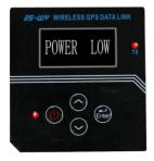
Sleep mode: If there is no any operation on the radio buttons for 10 minutes, the display will shut down to save power, the power indicator is still on, and TX indicator is still continue blinking. *Note: If the radio is in the sleep state, it is prohibited to press the power button to view the status of the radio, otherwise it will directly shut down.*
