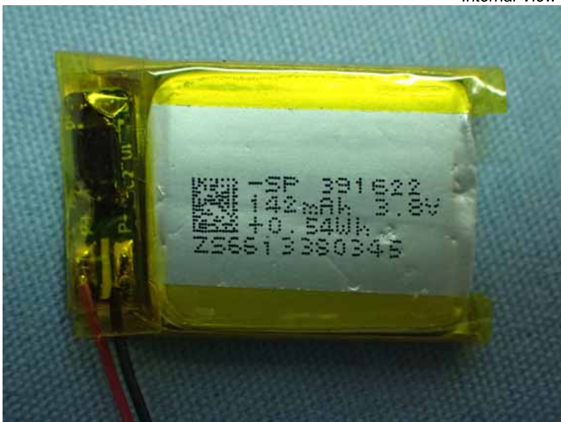
Figure 8 Internal View (Battery)
