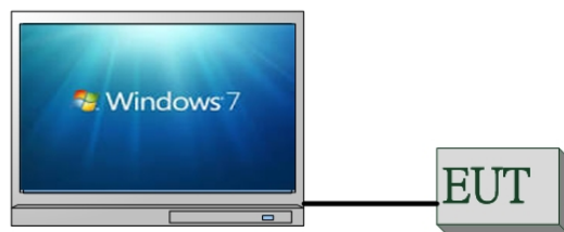
Fig.2-3 Conducted Emission (Antenna Port) Configuration
