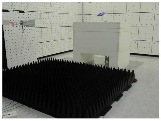
Radiated Emission Set up Photos (Front View of EUT)
