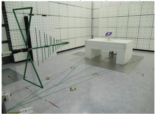
Radiated Emission Set up Photos (Above 1GHz)
