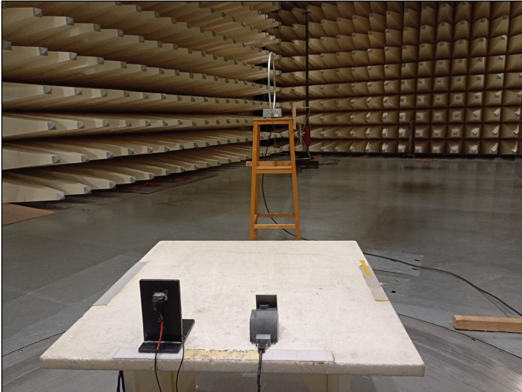
Photo 3: Setup radiated emission
