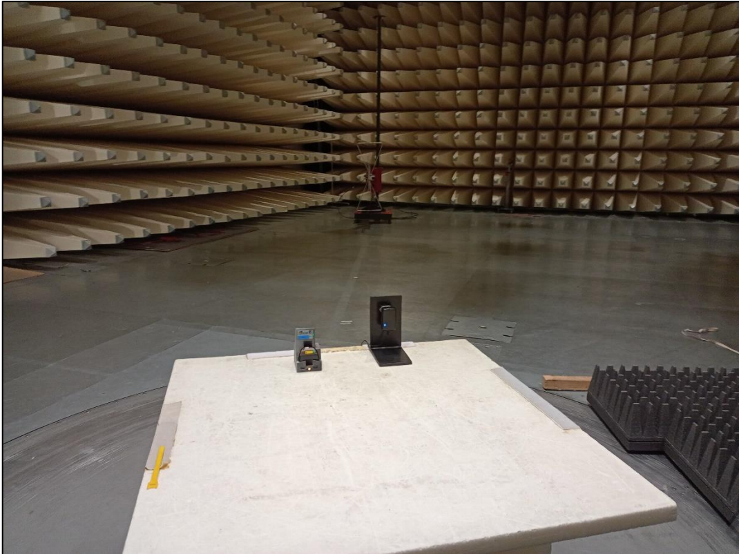
Photo 5: Setup radiated emission
