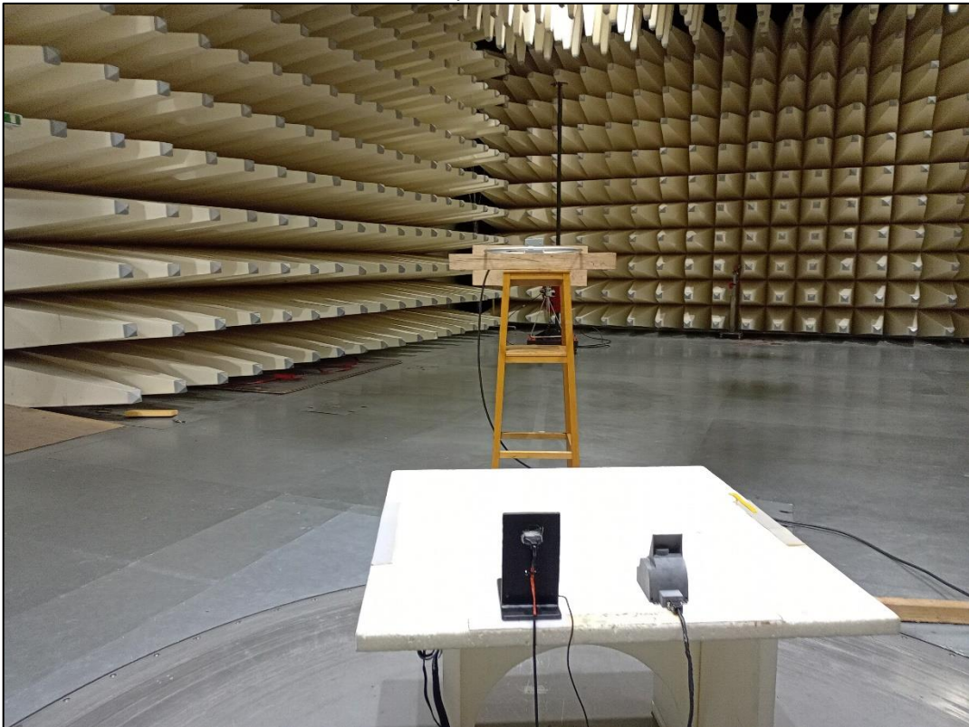
Photo 4: Setup radiated emission
