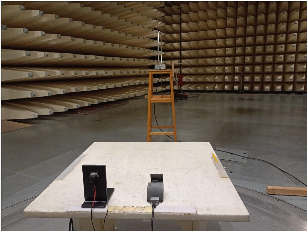
Photo 3: Setup radiated emission
