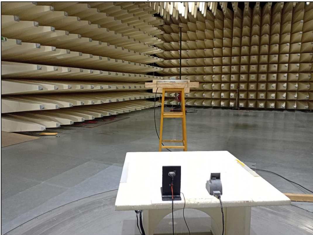
Photo 4: Setup radiated emission
