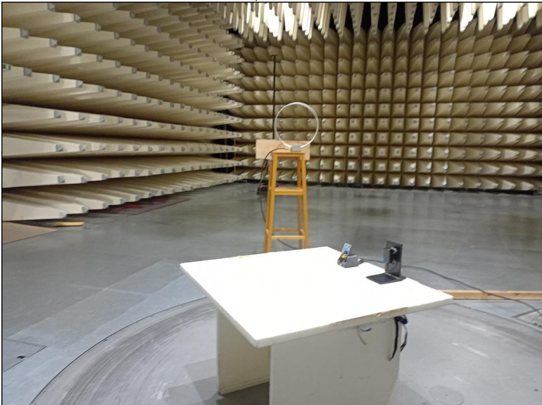
Photo 2: Setup radiated emission
