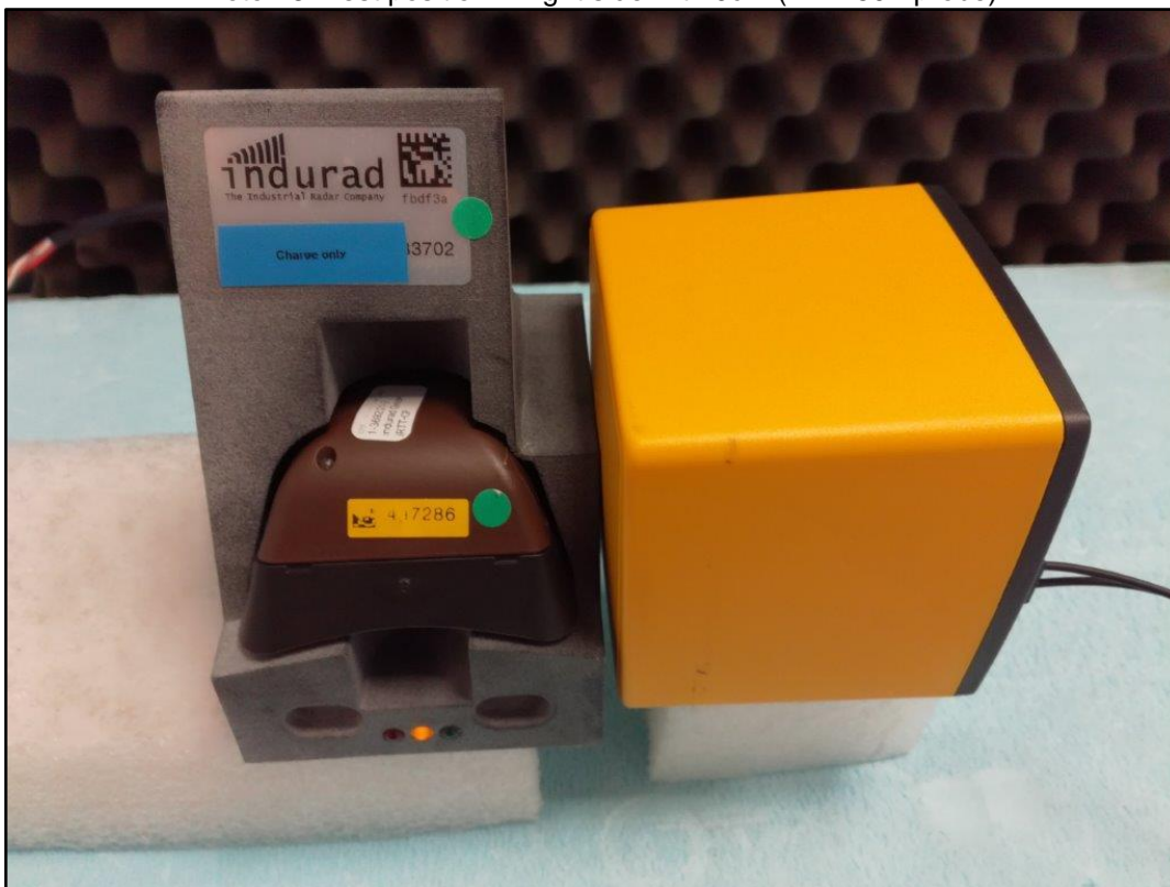
Photo 16: Test position - Right side with 0cm (EHP 50F probe)
