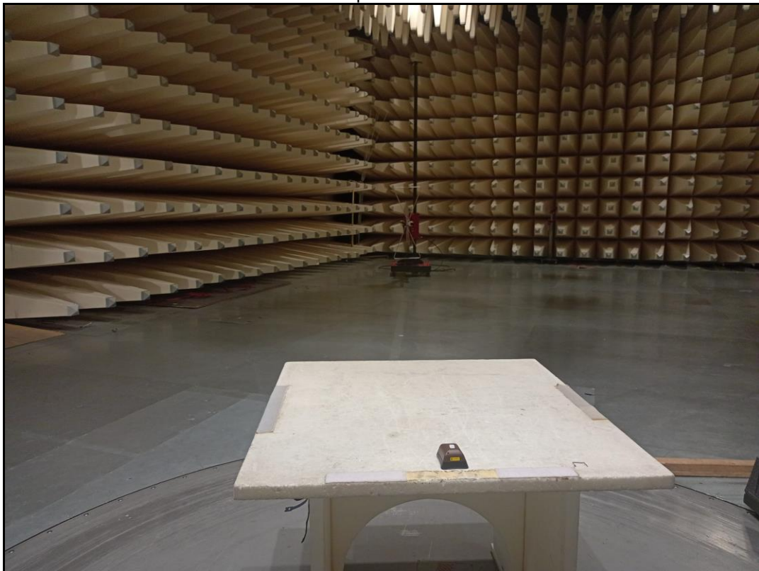
Photo 2: setup radiated emission
