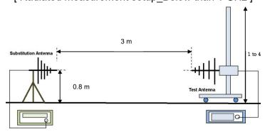
[ Effective Radiated Power measurement setup ]
