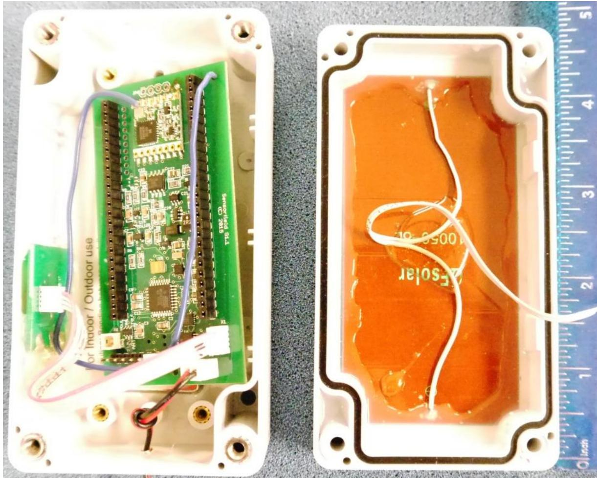
Note: Wiring leaving the enclosure is not on production units. This was used to facilitate testing.
