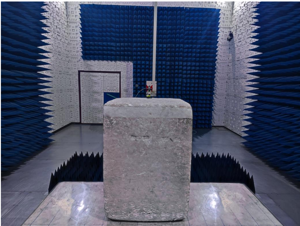
RADIATED EMISSION TEST SETUP ABOVE 1GHz
