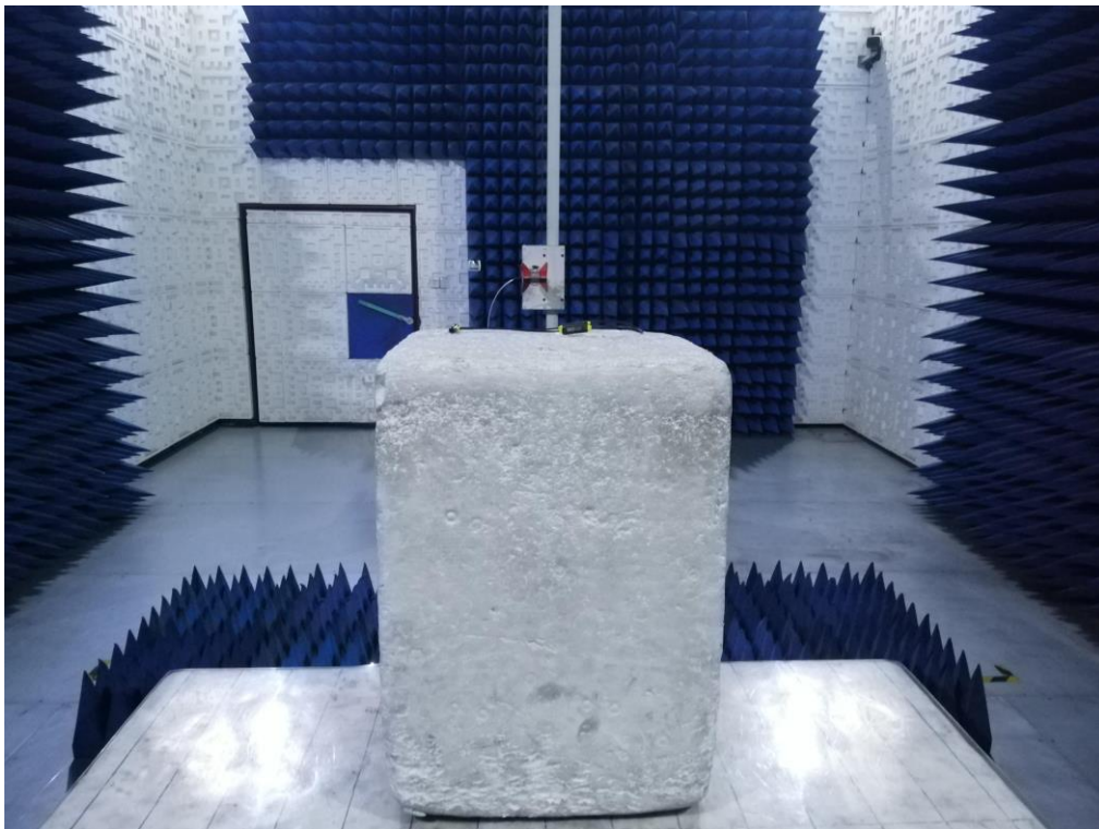
RADIATED EMISSION TEST SETUP ABOVE 1GHz
