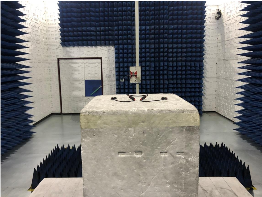
RADIATED EMISSION TEST SETUP ABOVE 1GHz
