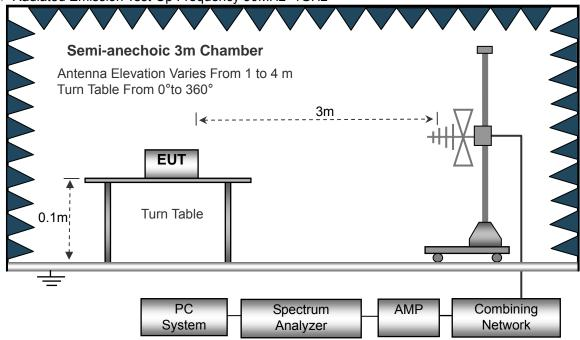
(C) Radiated Emission Test-Up Frequency Above 1GHz
