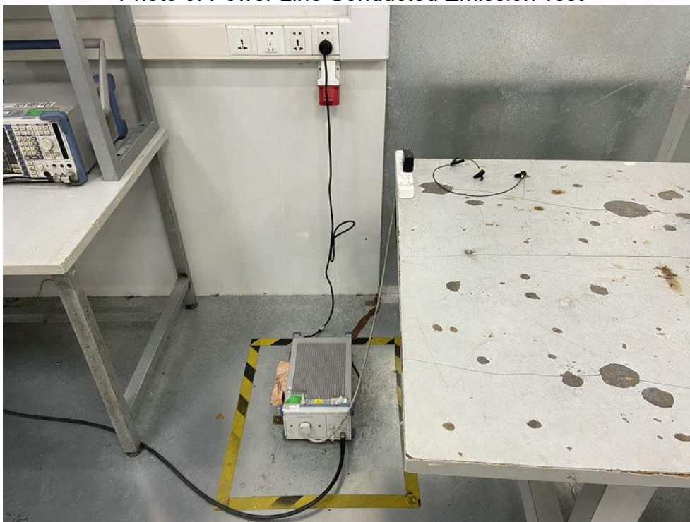
FCC ID: 2AJRD-ISOTUNES Photo of Power Line Conducted Emission Test
