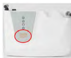
Figure 4: Magnet Inside Base Station
