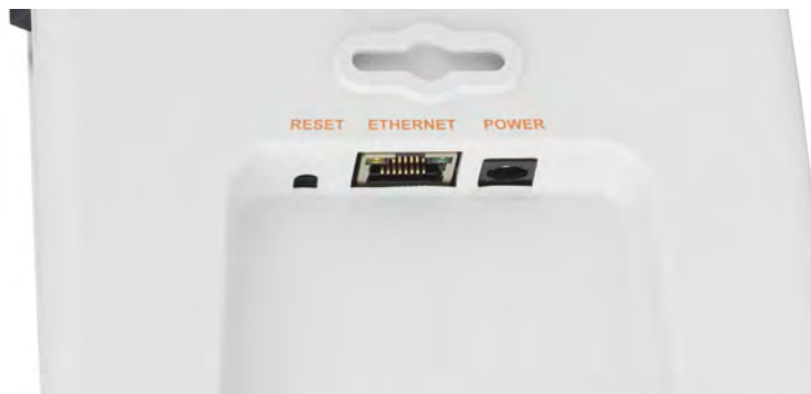
Figure 30: Base Station Connections
