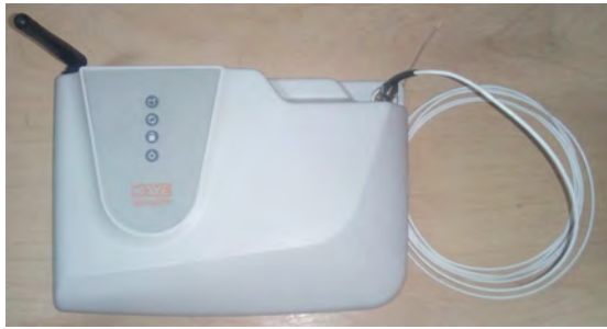
Figure 38: Base Station with Kayetenna
