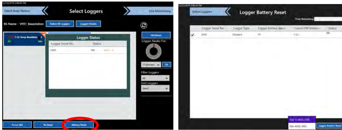
Figure 27: Logger Battery Reset
