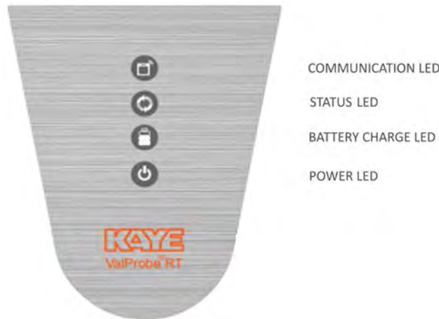
Figure 33: Base Station Status Panel
