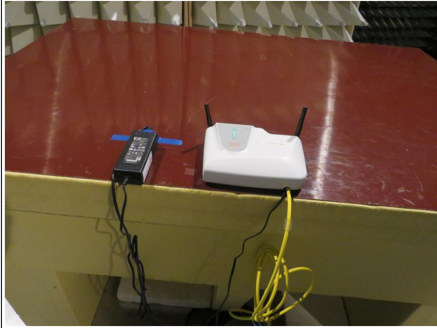
radiated emission - table setup with short antenna
