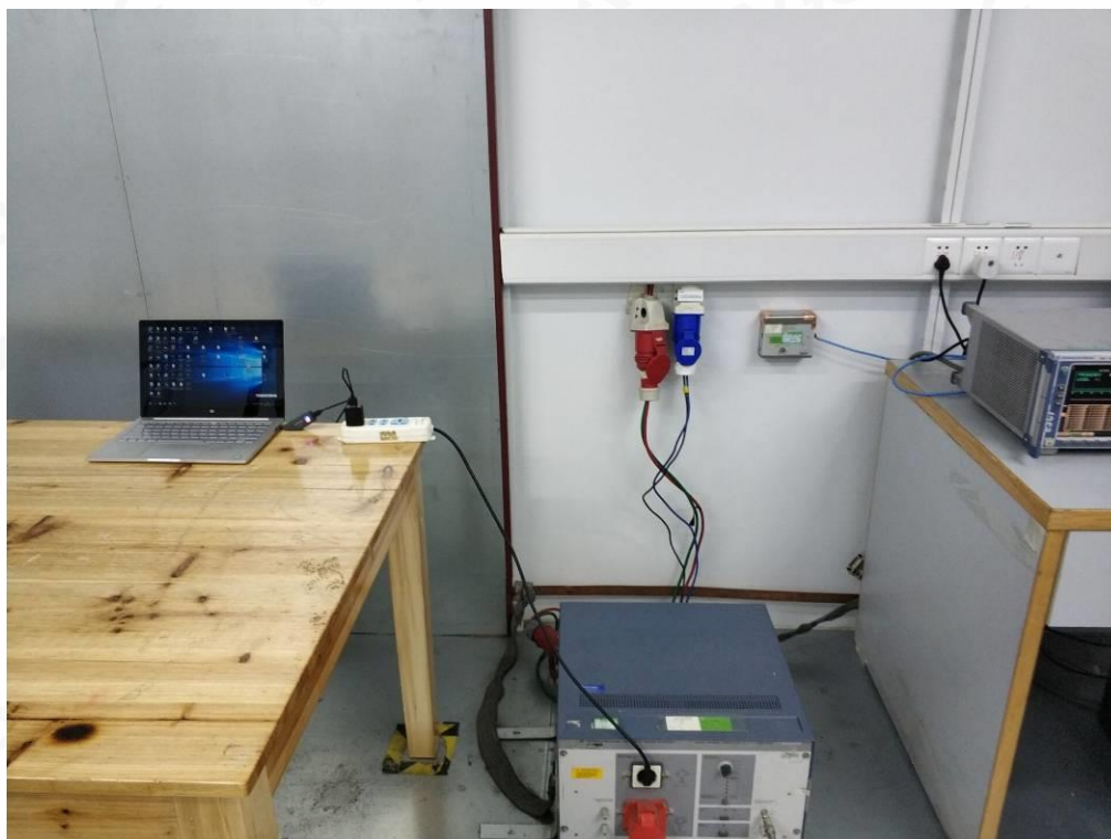
RADIATED EMISSION TEST SETUP BELOW 1GHZ
