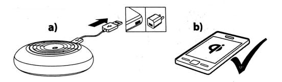
b. After connecting, the wireless charger will automatically start the load output and start the charging program. At this time, the wireless charger will automatically identify and charge the device with wireless charging function.
