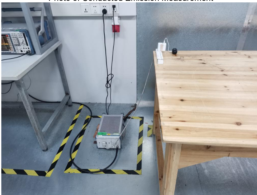
FCC ID: 2AJQ7TUNESMITH Photo of Conducted Emission Measurement
