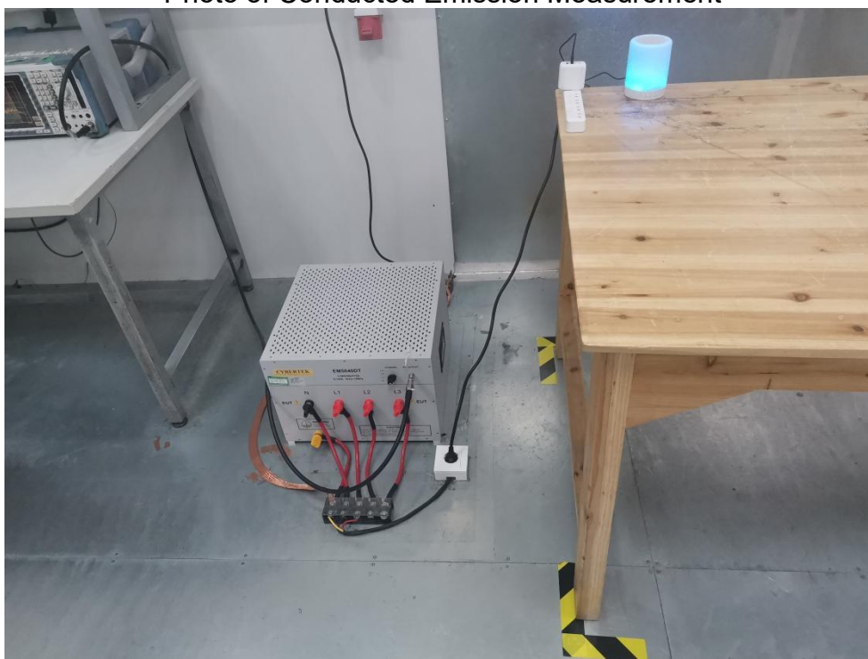
FCC ID: 2AJQ7TOUCH Photo of Conducted Emission Measurement
