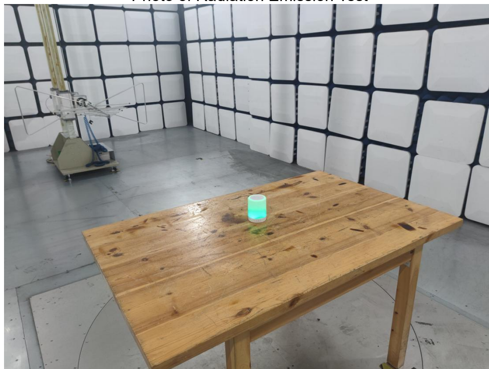
Photo of Radiation Emission Test
