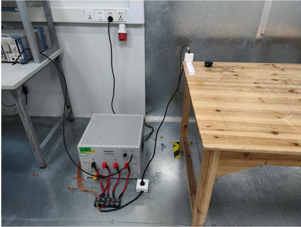
Photo of Conducted Emission Measurement
